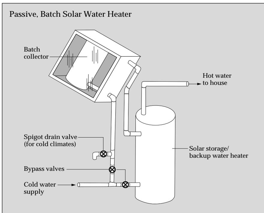
In a passive system, domestic water is heated in the solar collector, and transferred to the backup heater by the line pressure or thermosiphon action instead of by a pump.
